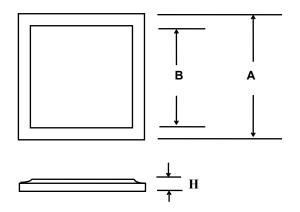
Bottom side metallization Ag thickness is 5KA minimum Top side metallization Al thickness is 25KA minimum Bottom side is cathode, top side is anode
